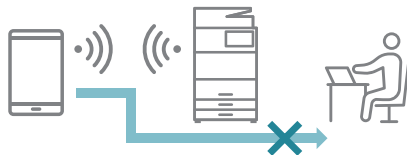
Mobile devices cannot access the company LAN via the MFP
